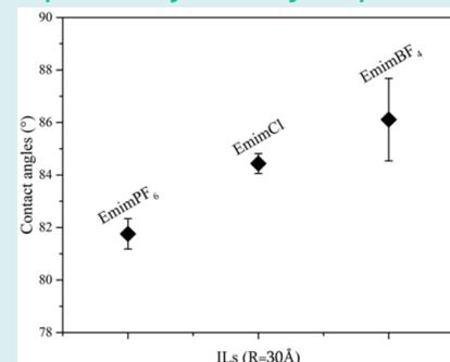
**Figure 2** The contact angles for hydrophilic ILs ([Emim][Cl] and [Emim][BF<sub>4</sub>]) and hydrophobic IL ([Emim][PF<sub>6</sub>]), the radius for ILs droplet is 30Å.
