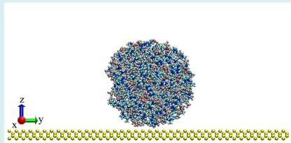
**Figure 1** Initial structure of the ensemble, the initial spherical droplet included 253 [Emim][BF<sub>4</sub>] ion pairs which radius of the spherical droplet is 25Å, the solid substrate with dimension of 76.8 × 153.6 × 5.76Å<sup>3</sup> consists of 3200 silicon atoms.
