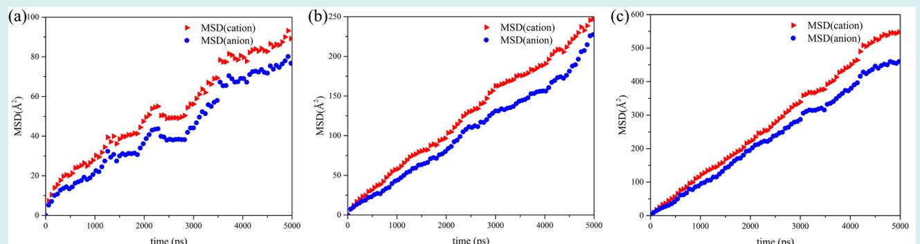
**Figure 4** The MSDs of imidazolium cations and anions for three ILs at t=400K, (a) represents [Emim][Cl], where (b) and (c) represent [Emim][PF<sub>6</sub>] and [Emim][BF<sub>4</sub>] respectively, the radius for all ILs droplets is 30Å.
