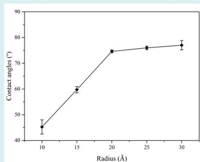
**Figure 1** The contact angles of [Emim][BF<sub>4</sub>] droplet with different radius on the silicon surface at the equilibrium state. Lines are drawn only for guiding purposes.
